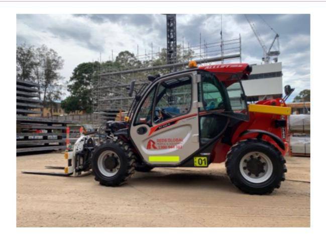
Model: MT-X 625 Comfort Load Capacity: 2500KG Max. Lifting Height: 5.85m
